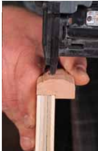
Here you can see what the shelf moulding looks like close up. Nail and glue the moulding to your plywood shelves.
