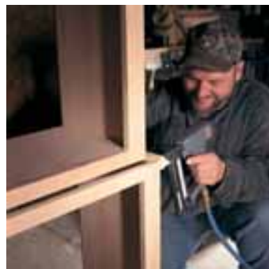
Attach the waist mould using nails. Nail it to the lower case and allow the top edge to cover the seam between the upper and lower cases.
